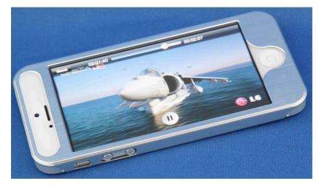
Eassee3D<sup>®</sup> technology is MADE IN GERMANY, with which you can watch 3D movies on all current iOS devices (iPhone / iPad). The system consists of the Eassee3D<sup>®</sup> app, that can be downloaded from the iTunes store, and the respective frame clip for the corresponding iPhone / iPad.
